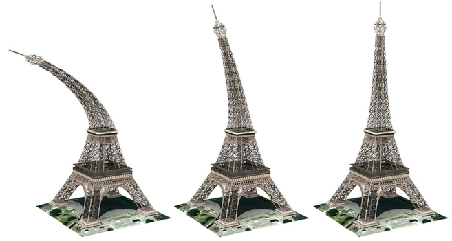
Fig. 4. Visualization of a co-rotational elastic deformation of the Eiffel Tower simulated with the stiffly accurate integrator.
